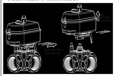
For reconnection, insert clip spring into clip adapter on actuator and push actuator onto valve to hear 'click'.
